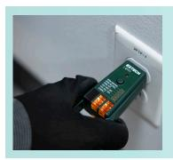
Rugged and affordable receptacle testers with convenient features like ergonomic pull bar and legend on both sides. These testers stand out due to their reliability, ease of use, and affordability. They are especially designed for detecting various wiring faults in electrical outlets. The ET11 comes with the ability to confirm the operation of GFCI circuits.
