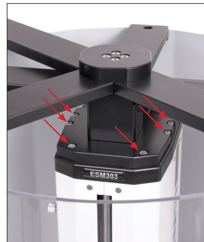
Fig. 1 Attaching the shield assembly to the ESM303 test stand column
