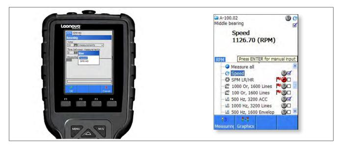
Recording is an Leonova function included in the platform. It allows the user to measure and record measuring results over longer periods of time, up to 50 hours. The recording function is an analysis tool which can show the interaction of various condition parameters over time.
