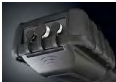
RFID measuring point identification
