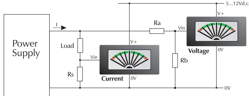
Simultaneous d.c. Voltage and Current Measurement.
