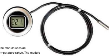
The EM32-1900 is an easy to mount LCD digital thermometer. The module uses an NTC temperature sensor to ensure high accuracy over a wide temperature range. The module uses an external sensor with a maximum temperature range of -40  $^{\circ}$ C (-40  $^{\circ}$ F) to +105  $^{\circ}$ C (221  $^{\circ}$ F).
