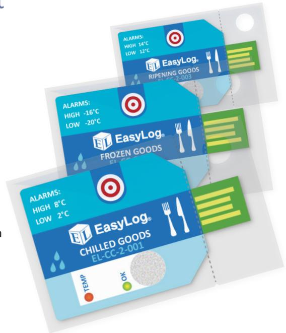
Each of the three Cold Chain loggers comes pre-configured for use in your particular application – simply press the button to start logging. During a logging session, pressing the button will light up the status LEDs to give a quick indication as to whether the temperature has exceeded an alarm condition at any point.
