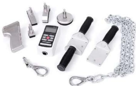
Thank you for purchasing a Mark-10 Series E Ergonomics Kit. Please read through this Quick Start Guide and the complete force gauge User's Guide before using this kit.
