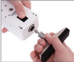
Attachments are mounted to the gauge's receptacle via the Click-Lock™ mechanism. Line up the attachment with the receptacle, and press in until a click occurs. The attachment may be inserted in 90- or 180-degree orientations. To release the attachment, pull back on the lever in the rear of the housing, as shown at left.
