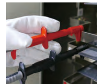
For clamping around the target busbar
