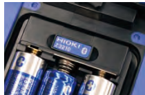
Attach to enable Bluetooth® wireless technology
