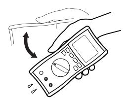
Securely hold the instrument with the drain holes away from you and shake it approximately 20 times until no water drops are coming out.
