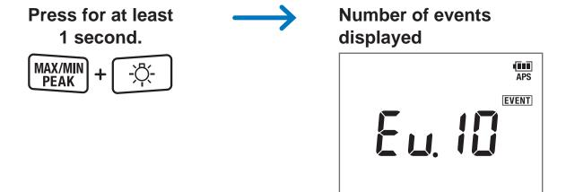
An event with a duration time of less than 200 ms may not be accurately measured, failing to detect the event.
