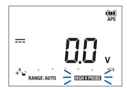
3 Connect the P2000 DC High Voltage Probe to the measurement terminals of the instrument.
