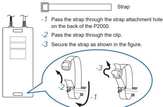
3 Attach the strap buckle to the strap holes (bottom) of the instrument and connect it to the clip that you attached to the P2000 with the strap.
