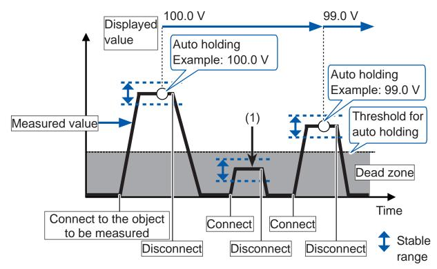
(1) Not retained automatically (the threshold is not exceeded).
