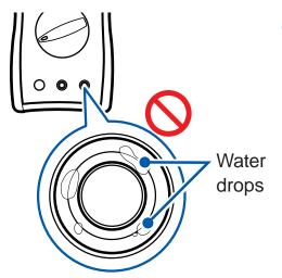
4 Check that there are no water drops inside the measurement terminals.
