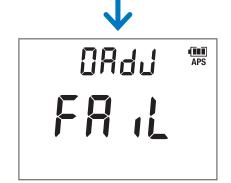
Screen displayed when zero adjustment fails
