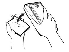
Securely hold the instrument with the measurement terminal facing down and gently tap the instrument against a soft cloth, etc. approximately 10 times until no water drops are coming out.
