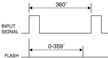
**NOTE:** If the input signal frequency exceeds upper or lower limits, the alarm dashes (----) will be displayed or the strobe will stop flashing.
