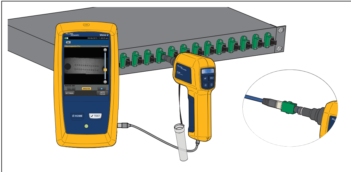
Figure 48. Inspect an Endface (FI-3000 shown)
