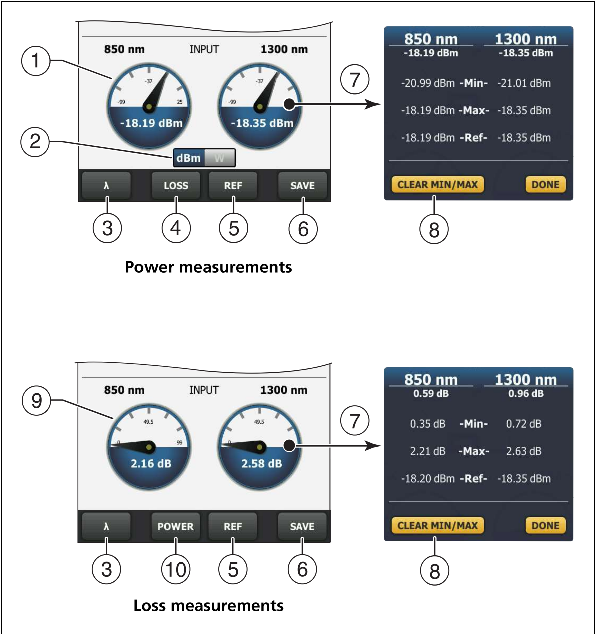
Figure 123. Power Meter Measurements and Controls
