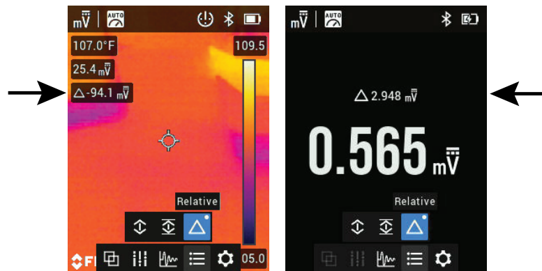
Figure 10.19 Relative mode menu from the thermal image mode (left) and multimeter mode (right). The arrows show where the reference value is shown.
