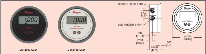
The Dwyer Series DM-2000 Differential Pressure Transmitter senses the pressure of air and compatible gases and sends a standard 420 mA output signal. The DM-2000 enclosure is specifically designed to mount in the same diameter cutout as a standard Magnehelic® gage. A wide range of models are available factory calibrated to specific ranges.
