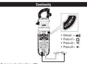
$\bullet$  Buzzer sounds at less than  $<40\Omega.$
