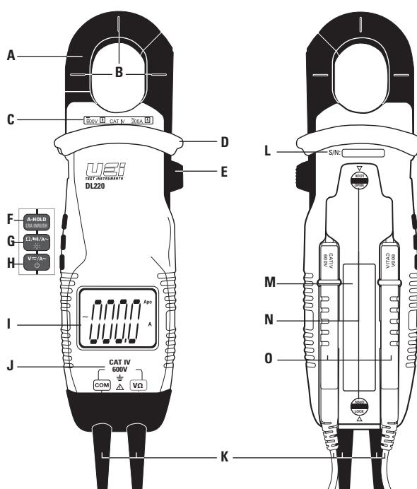
**A. Clamp:** Measure inductive AC current. Opens to 0.76" (19.10mm).
