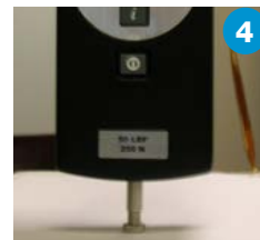
Apply Push Force Apply a pushing force to the sample under test. Observe the load bargraph (fills from the center towards the “C”) and the Compressive Load Indicator (arrows). The main display will indicate the load being applied to the load sensor shaft using the fixture/adapter.
