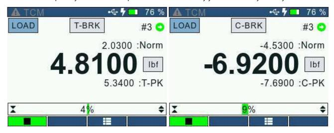
The DF3 Series gauge will report the following as part of a Break Detect test:
