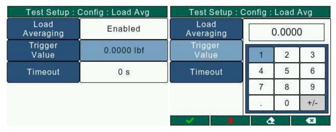
The user will have to exit the Configuration (ConfigurationScreen.html) screen and save changes for the Preload value setting to be applied.
