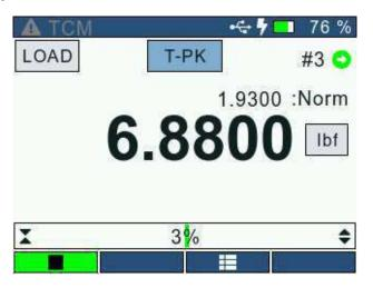
When the gauge is in Peak Tension mode (T-PK), the gauge will display the maximum tensile load that was measured by the loadcell sensor. In addition to that, the user will also be able to view the Peak Tension value as a sub-reading when the gauge is in Normal or Tension Break (T-Brk) (BreakDetection.html) Mode.
