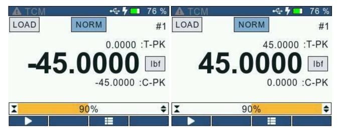
When the applied load is greater than **90%** of the maximum range, the load bar graph is **Red** in colour.
