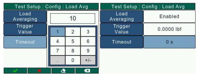
The user will have to exit the Configuration (ConfigurationScreen.html) screen and save changes for the Timeout setting to be applied.
