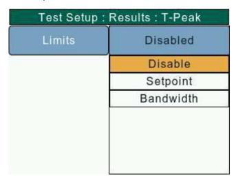
Pass/Fail limits can be configured from the Test Setup: Results (TestSetupResults.html) screen. This screen allows the user to select a particular result and configure the Pass/Fail limit as per requirement. The Pass/Fail limits can be disabled or set using either the Setpoint or the Bandwidth method.
