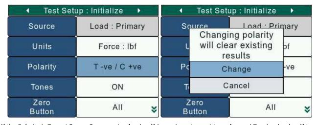
If the Polarity is T -ve / C +ve, Compression loads will be assigned a positive value and Tension loads will be assigned negative values.
