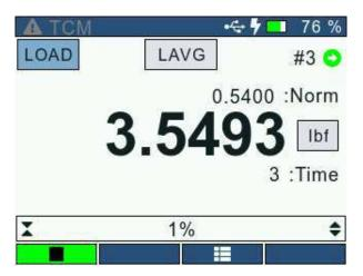
This load averaging test works identical to the Force-Based method except it adds "Time" as a factor. You may set the Timeout Value from 1 second to 3600 seconds. The gauge will begin to collect and average the measured values once the "Preload Value" has been sensed. The gauge will continue to average until the measured load drops below the preload value OR until the specified time has elapsed. When the test is completed, the gauge will display the "Average Load".
