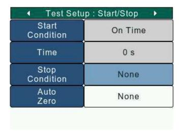
If the Stop condition is set to 'On Time', the user gets to set the test duration. The stop timer is visible on the Home (HomeScreen.html) screen indicating the time left in seconds. The user can enter a value between 0 - 3600 s as the stop duration.
