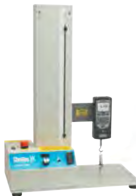
DFS II gauge mounted to LTCM100 tester
