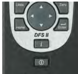
Shown: The power On/Off button is located on the front of all DF II Series force gauges.
