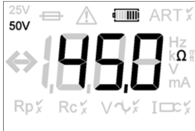
Figure 14: example two-terminal resistance reading (DET4 display shown)
