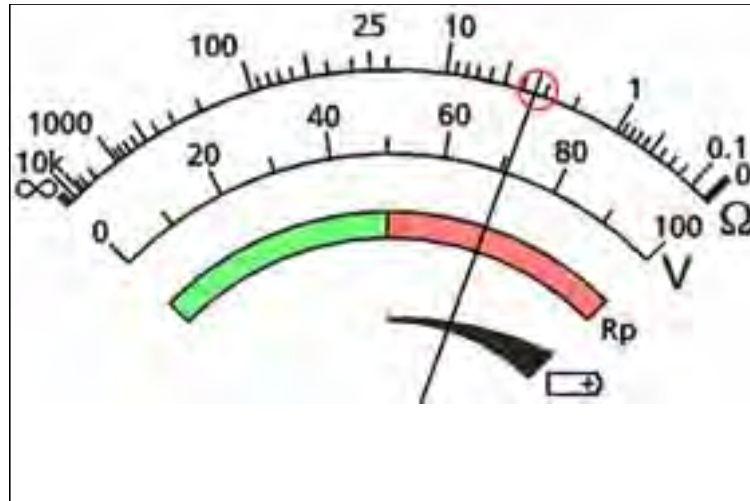
Figure 17: example two-terminal resistance reading
