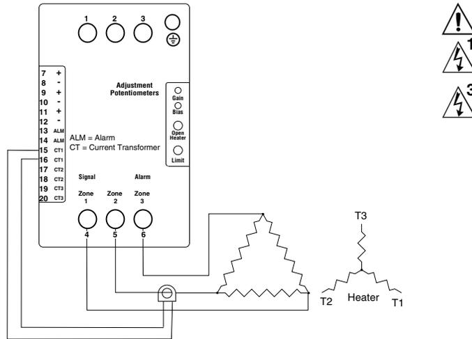
**3-phase, 3-leg Alarm, Shorted SCR and Open Heater Alarm**
