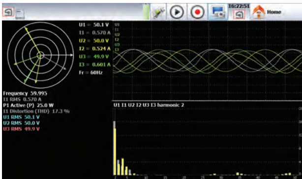
Real time display of Fresnel diagram, oscilloscope mode and harmonics (up to 50th)
