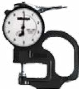
Testex replica tape can be used with a gage to measure the surface roughness ("profile") of blast-cleaned steel in the roughness range 0.8 to 4.5 mils (or 20 to 115 micrometers). Because inspectors, as a rule, have a target profile in mind, it is always best to start measurements with the grade of tape that has the target profile closest to the center of its range. Each grade of replica tape is most accurate near the center of its specified range.
