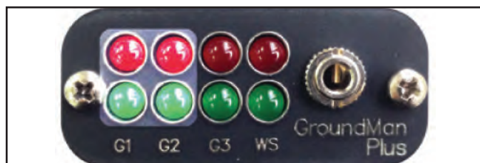
Figure 3. LED lights used to set resistance alarm level.
