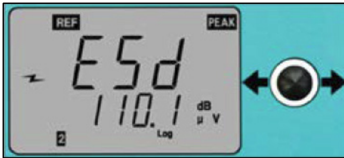
Figure 7. Modifying the ESD event threshold
