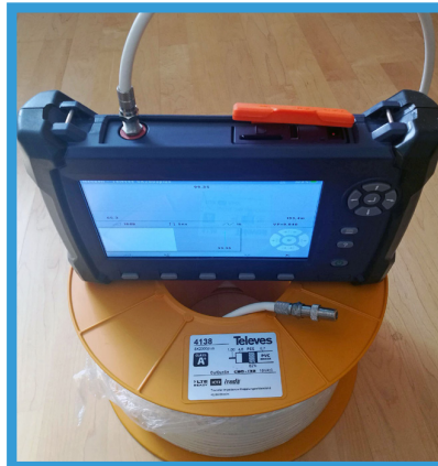
Figure 4: An important application of the CS90 is the preliminary testing of a cable drum for correct length and homogeneous impedance curve
