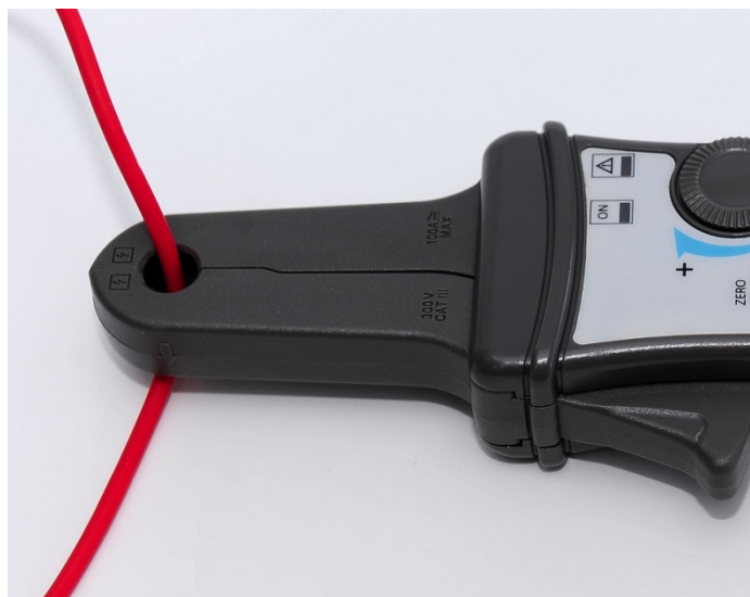
Figure 5: Connecting the CP62 current probe.
