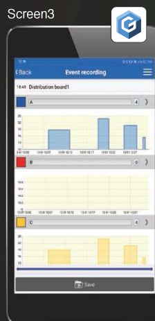
Visualize intermittent GFCI and RCD trips Review trip times and maximum current values
