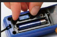
Attach to enable Bluetooth® wireless technology
