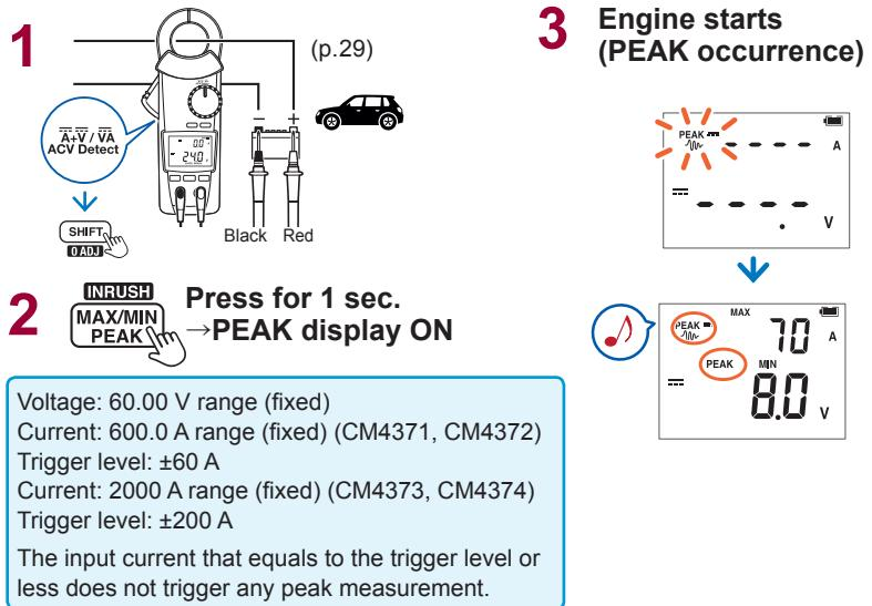
Simultaneous display of DC current/voltage peak values
