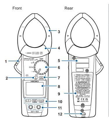
1 Operation grip 2 Fn key (Selects function indicated in blue lettering) 3 Jaws (p.32) 4 **Barrier** 5 Serial number (The serial number consists of 9 digits. The first two (from the left) indicate the year of manufacture, and the next two indicate the month of manufacture.) Rotary switch 6 7 **HOLD** key LCD 8 9 Battery cover 10 Operation keys 11 Measurement terminals 12 Strap hole
