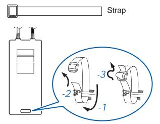
3 Attach the strap buckle to the instrument and connect it to the clip that you attached to the P2000 with the strap.
