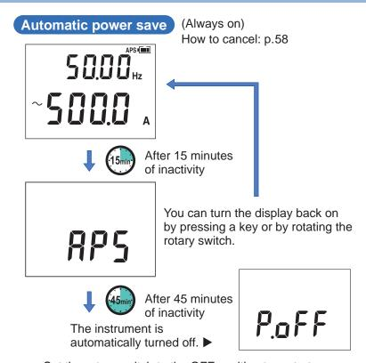
Set the rotary switch to the OFF position to restart.
