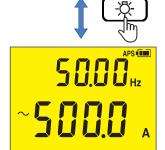
Backlight on Automatically shut off after 40 s of inactivity (Automatic shutoff is always enabled) How to cancel: p.59
