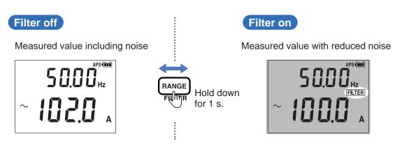
Frequency characteristics when the filter function is enabled (100 A input)
