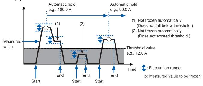
Suppose that the measured value has fallen below (voltage, current) or exceeded the threshold value (resistance, continuity check, diode) after the displayed value froze. When the two auto-hold conditions are met again after that, refreshing measured values will stop.
