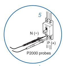
Connect the P2000 DC High Voltage Probe to the measurement terminals of the instrument.
