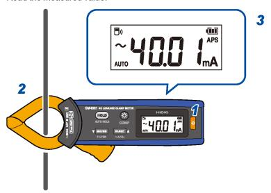
4 Press the RANGE key for 1 s or more to switch between current measurement and frequency measurement.
