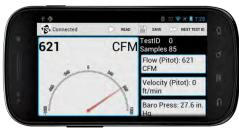
Utilizing wireless Bluetooth® technology, this app for Android™-based smartphones and tablets communicates with the instrument remotely over 100 ft. (30.5 m) away and displays sample data in real time. Attach comments, voice notes, and photos to test ID data for export via email to generate reports.
