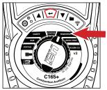
Rotate the selector dial to **PRS/TEMP.**
