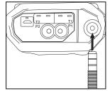
Once complete, remove probe from stack, allow analyzer to purge in fresh air until CO sensor readings return to ZERO (0) and O2 readings reading return to 20.9%.
