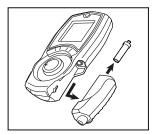
Remove protective rubber boot. Remove water trap from analyzer. Remove particle filter from water trap and replace with new one. Reattach trap and boot.
