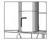
Place combustion probe or true draft probe tip in the flue to measure draft.
