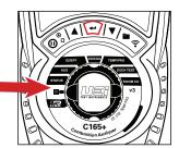
The **AUX** screen allows you to assign any of the following parameters on any display line. CO2, CO, NO (if fitted), NOx (if fitted), O2, TF, Ti, Ta, Delta (Δ), Loss, EFg, Xair, Ra (CO/CO2 Ratio), PI, Fuel Type, PRS or Blank.
