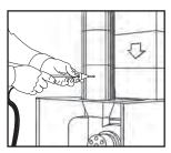
Remove the probe from the flue and allow analyzer to purge with fresh air until readings return to zero. O2 to 20.9%
