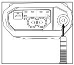
Insert Flue probe into stack. Adjust cone so end of the probe is approximately at the center of the stack.
