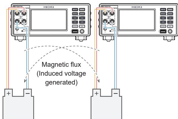
Simultaneous measurement can result in mutual interference due to electromagnetic induction.
