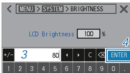
3 Use the numerical keypad to enter the backlight-brightness level.
