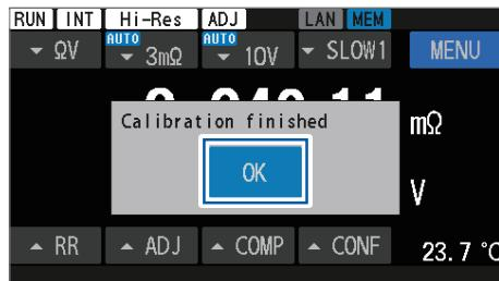
4 After the calibration processes are completed, tap **[OK]**.
