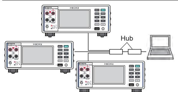
In addition, after creating a program, connecting external equipment, such as a computer to the communications command port using TCP allows you to control the instruments through communications commands. See Communications Command Instruction Manual for details.
