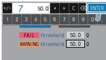
7 Use the numerical keypad to enter the warning threshold.
