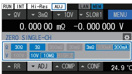
Ranges with obtained adjustment values are displayed in blue, while shaded areas indicate ranges without obtained adjustment values.
