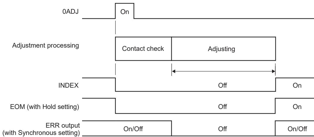
The ERR signal turns off upon successful zero adjustment and turns on if the adjustment fails. If the 0ADJ signal is input during a measurement, the instrument suspends the measurement, starting single-mode zero-adjustment.
