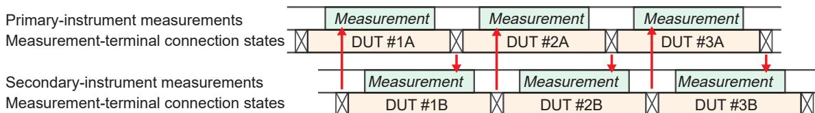
**If the connection state on either line changes during a measurement on the other line, the effect of mutual interference cannot be eliminated.**
