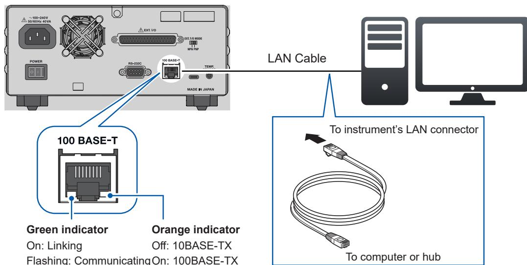
If the green indicator fails to light up after connecting the instrument to the LAN, there may be a malfunction in the instrument or connected devices, or the LAN cable may have a break or a poor contact.
