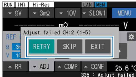
(When repeating the adjustments on failed channels)
