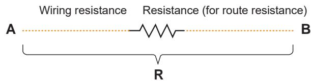
Prepare a calibration cable as shown in the figure above, and use a high-precision resistance meter to determine the resistance value of the resistance  $R$  between A and B.
