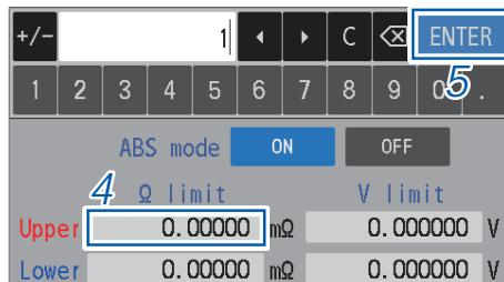
4 Under [ $\Omega$  limit], tap the [Upper] box and use the numerical keypad to enter the resistance upper-limit value.
