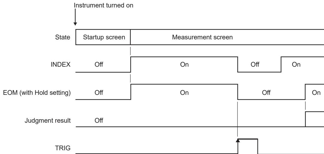
Judgment results: R\_HI, R\_IN, R\_LO, V\_HI, V\_IN, V\_LO, R\_R\_PASS, R\_R\_WARNING, R\_R\_FAIL, PASS1, FAIL1, PASS2, and FAIL2, including ERR
