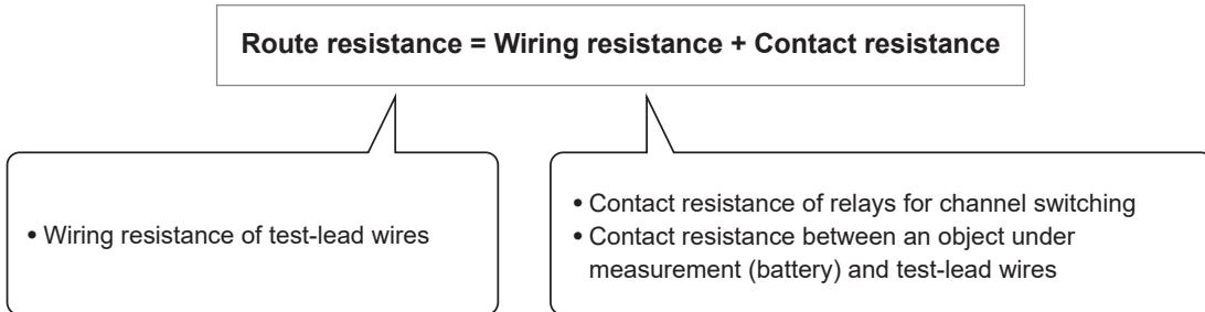
The route resistance is measured simultaneously with the internal resistance of a battery. Continuous monitoring of the route resistance allows effective maintenance management of a measurement system. Additionally, thresholds can be defined for route resistance measurement, enabling a three-level judgment (Pass, Warning, and Fail).
