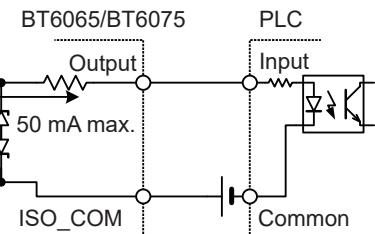
Connection with PLC input (negative-common)
