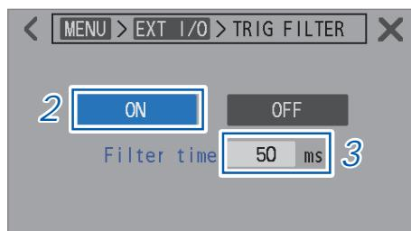
2 Tap **[ON]** to turn the filter capability on.
