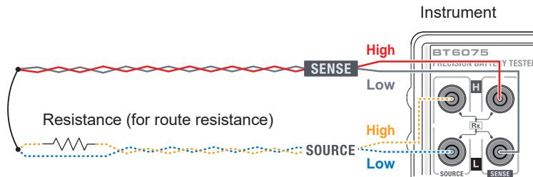
At this time, use the assembled calibration cable for a terminal to be calibrated (in the figure, Source Hi).
