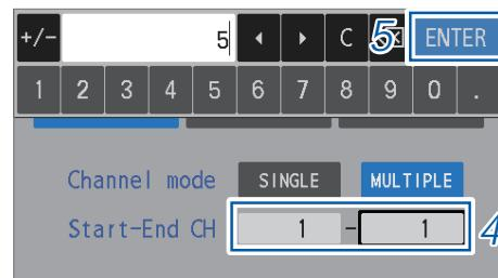
4 Use the numerical keypad to enter the start and end channels for the referential adjustment.
