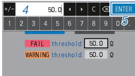
4 Use the numerical keypad to enter the fail threshold.
