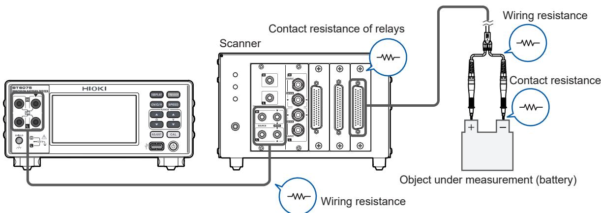
The four-terminal route resistances ( $R_{\text{Source Hi}}$ ,  $R_{\text{Source Lo}}$ ,  $R_{\text{Sense Hi}}$ , and  $R_{\text{Sense Lo}}$ ) are defined as follows:
