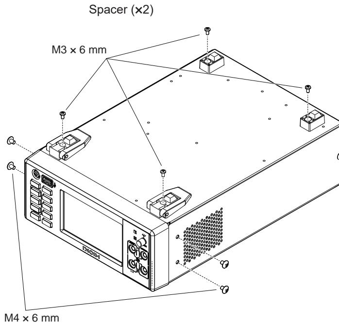
**1** Place the instrument with its bottom face up and remove the eight screws on the support feet and its sides.
