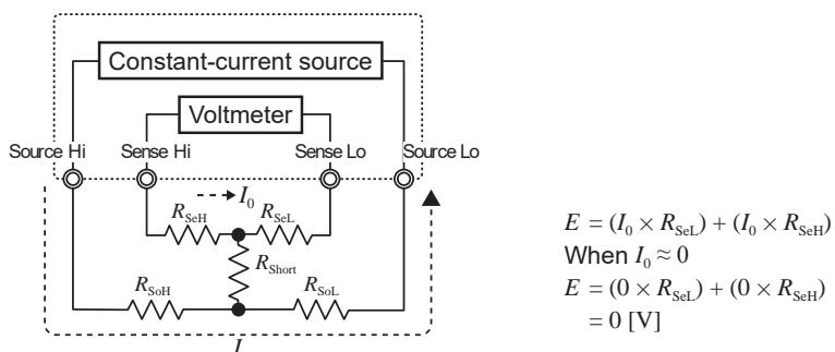
First, short-circuit between Sense Hi and Sense Lo to set the voltage between them to  $0 \text{ V}$ . The wire resistance of the test-lead wires used ( $R_{SeH} + R_{SeL}$ ) should not exceed several ohms. The current  $I_0$  minimally flows through the Sense terminals, which are the voltage measurement terminals. If the test-lead wires have a resistance of several ohms, the voltage between Sense Hi and Sense Lo will be almost zero.
