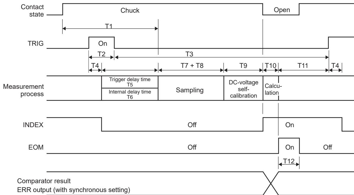
(3) When the trigger source is set to [INT], the trigger-reception continuation mode is set to [ON], and the DC-voltage self-calibration is set to [AUTO]
