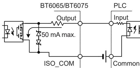
Connection with PLC input (positive-common)
