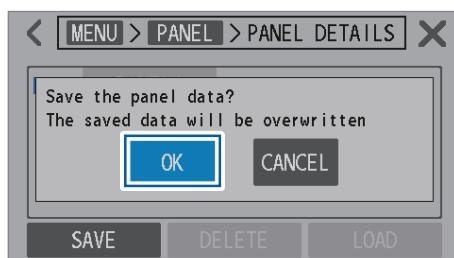
3 To overwrite the existing measurement conditions with the present ones, tap [OK].
