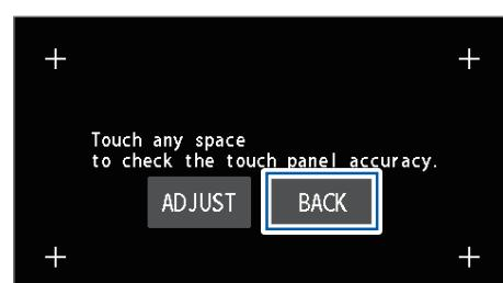
5 Tap any point to check for inaccuracies in the tapped position.
