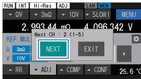
The next channel and the channels to be measured are displayed.
