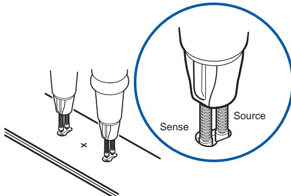
The pin-supporting part has a protruding line on the Sense side. Face these lines in the same direction when performing zero adjustments. Select two holes on the 0 Adj Board arranged symmetrically with respect to the line through the center plus sign, ensuring they are positioned at approximately the same distance as the terminals of the battery under measurement, then press the pins against the bottom of the holes.
