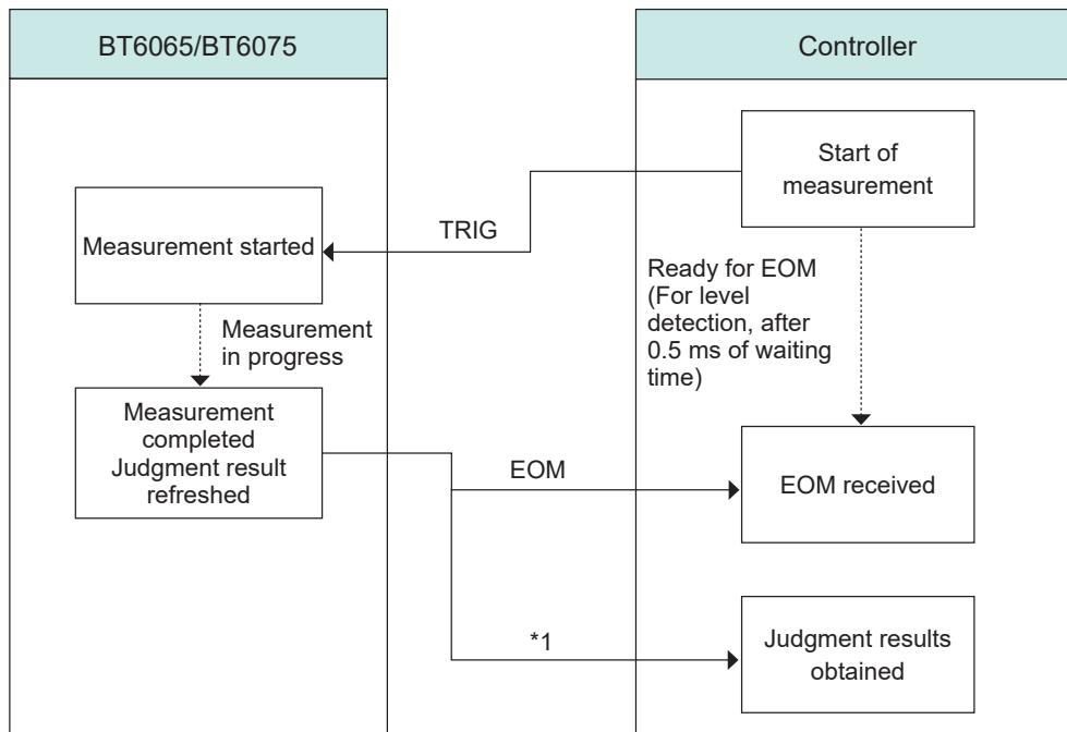
\* 1. R\_HI, R\_IN, R\_LO, V\_HI, V\_IN, V\_LO, R\_R\_PASS, R\_R\_WARNING, R\_R\_FAIL, PASS1, FAIL1, PASS2, FAIL2, and ERR
