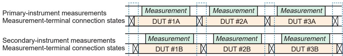
**During measurement on either line, the connection state on the other line remains unchanged.**
