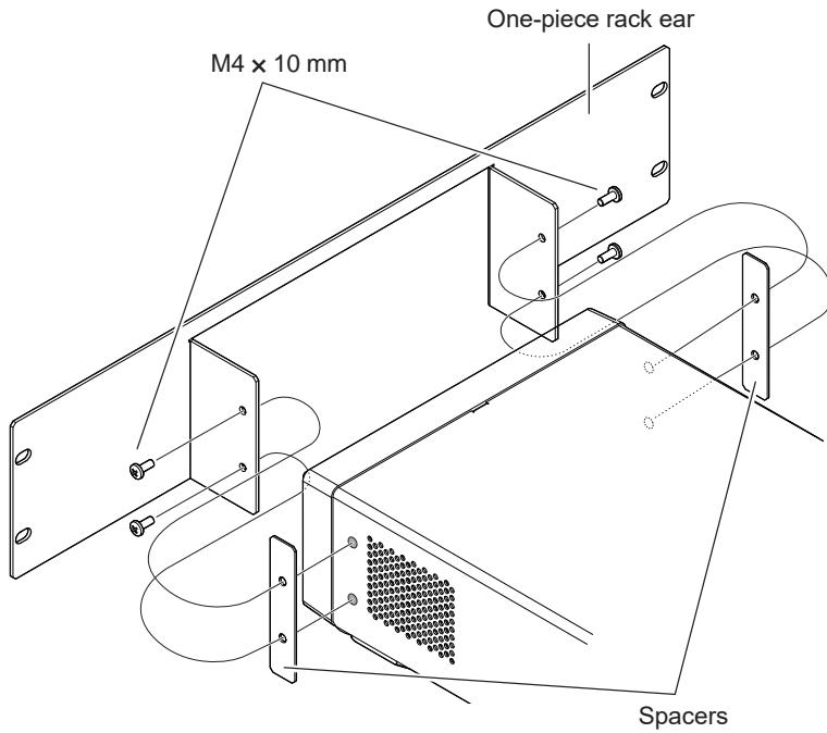
**3** Insert the spacers between the rack-mounting ear(s) and both sides of the instrument and attach the ear(s) with the specified screws (four in total).
