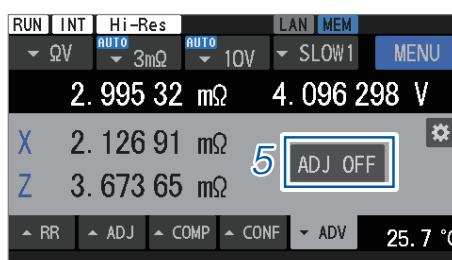
The reactance (X) and impedance (Z) of the object under measurement are displayed.
