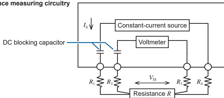
$R_1$  to  $R_4$ : Resistance of the test-lead wires and contact resistance of contact points
