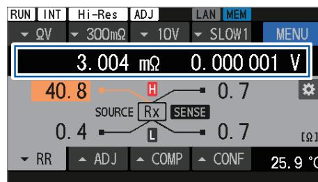
When the measured value exceeds the fail threshold
