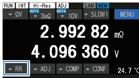
1 While making measurement with the resistance measuring function ([ $\Omega$ V] or [ $\Omega$ ]), tap [RR] or press the DISPLAY key.
