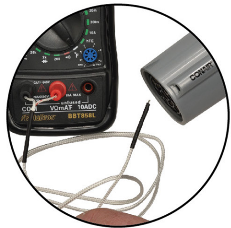
Includes K-type temperature thermocouple
