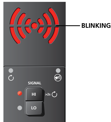
Figure 3.1b: Transmitter indicator showing signal in HIGH mode
