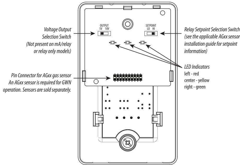
The voltage output selection switch is only available on voltage output models. For mA/relay output and relay only models, this space is empty.
