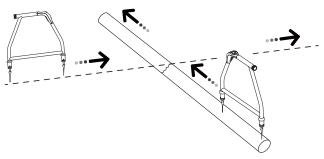
If it is suspected that there is just one fault, insert the A-frame approximately 3 ft (1 m) from the ground stake. Note the two digit number - this is approximately the maximum reading that will be measured over the fault.
