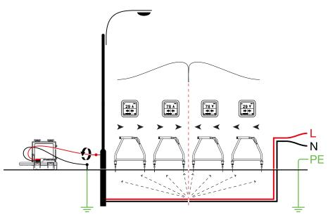
7. Carefully place the A-Frame before and after the fault to pinpoint it. Repeating this in a line perpendicular to the direction of the cable will pinpoint the fault laterally.
