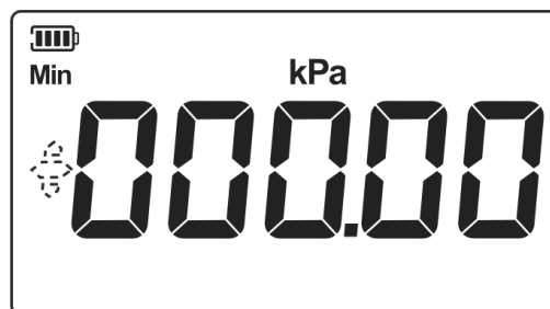
Figure 14 Lower limit calibration point
