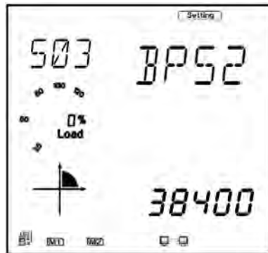
Figure 5-53 Baud Rate setting for the AXM-RS485 module
