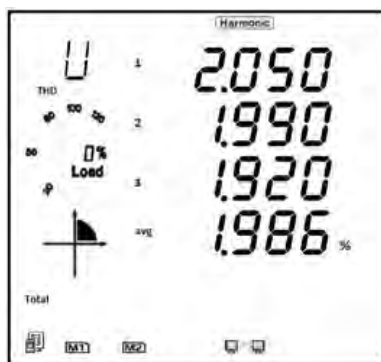
Figure 3-21 - Harmonic Distortion Reading
