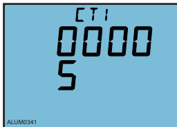
Fig.3-44 CT primary side ratio setting
