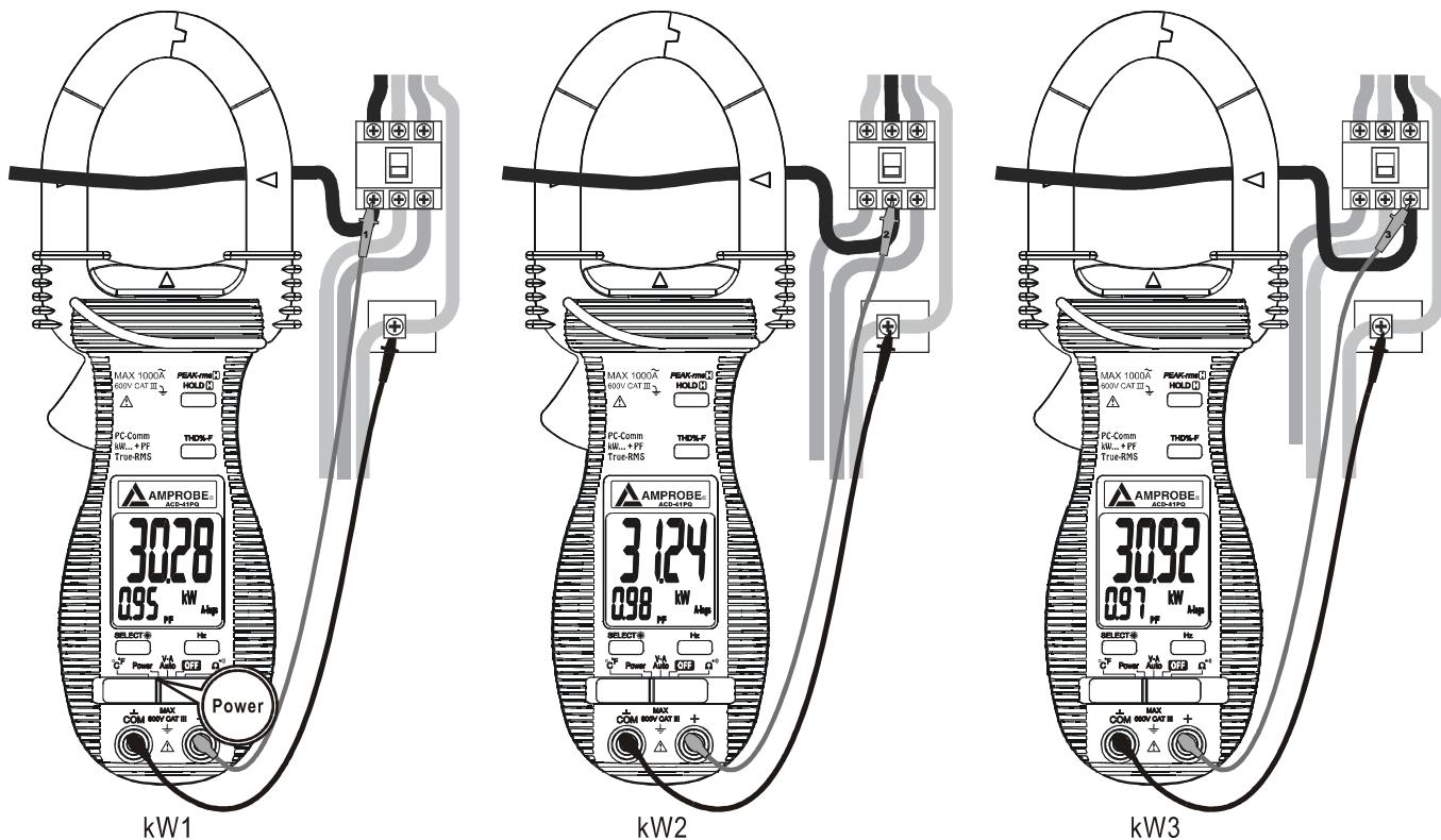
In both un-balanced and balanced load cases, 3-Phase 4-Wire ( $3\sim 4W$ ) systems, measure the phase-to-neutral powers  $kW_1$ ,  $kW_2$  and  $kW_3$  of each phase separately as illustrated. System (total) power  $kW_{\text{Total}}$  is the summation of all three phase-to-neutral powers. That is:
