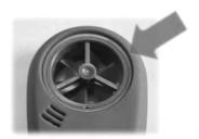
Step two: Remove sleeve by pulling it over the top of the ABM-200 and off of the bottom.
