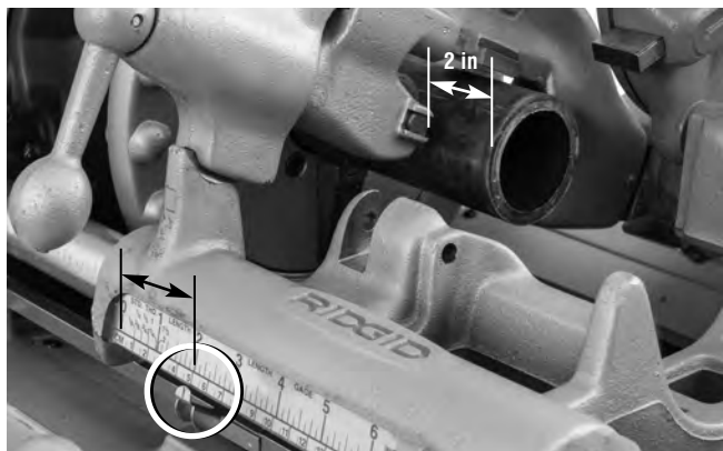
Figure 20B – Length Gauge Pointer At Desired Length
