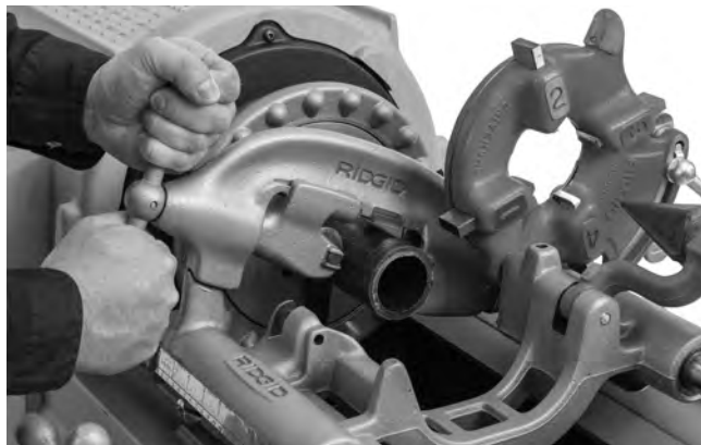
Figure 21 – Cutting Pipe with Cutter
