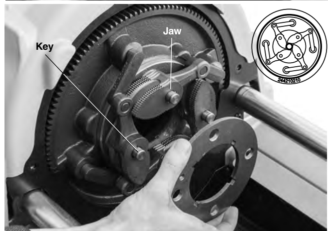
Figure 32 – Changing Auto Chuck Machine Jaws
