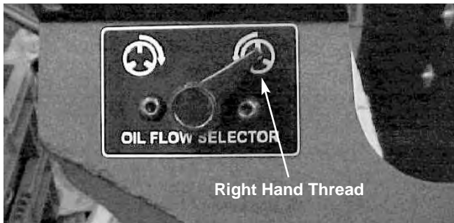
Figure 24 – LH or RH Oil Flow Selector
