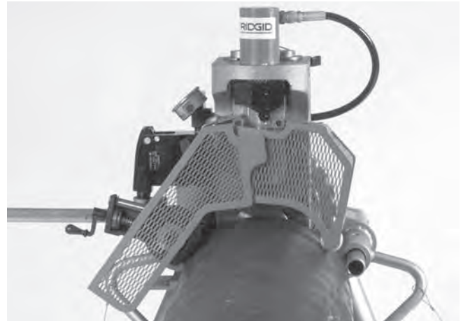
Figure 14 – Guards in the Operating Position
