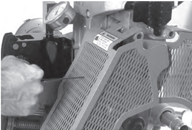
Figure 18 – Loosening Set Screw In Upper Roll Housing
