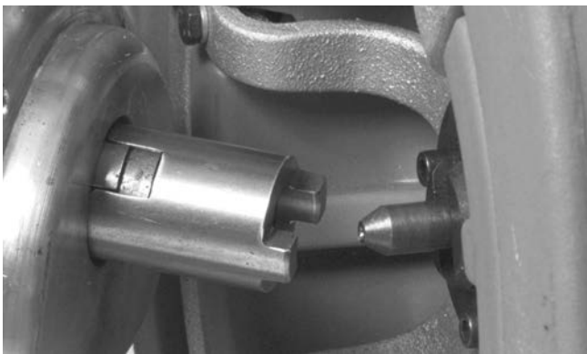
Figure 15 – K-3800 Drum with K-6200 Adapters
