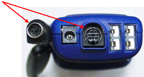
“D” Shaped mini-DIN connector
