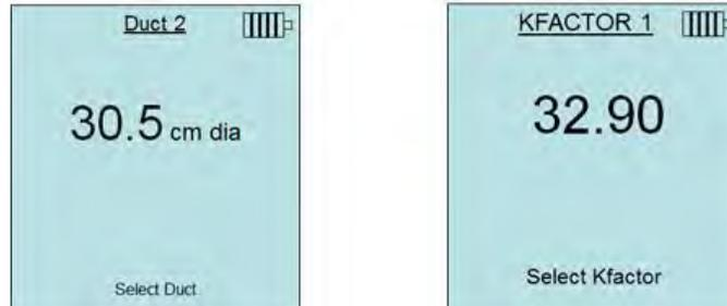
Make adjustments with the ▲ or ▼ arrow keys and press ← to accept, or enter the **Select Duct** or **Select Kfactor** menu to choose a different pre-programmed flow value or dimension.
