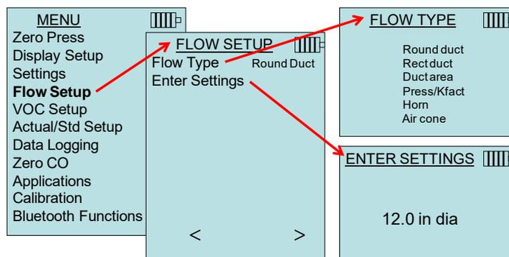
**Round duct, Rect duct** and **Duct area** are used to perform a duct traverse using a pitot probe or thermoanemometer probe. For more information on how to perform a duct traverse, refer to [Application Note TSI-106](#).
