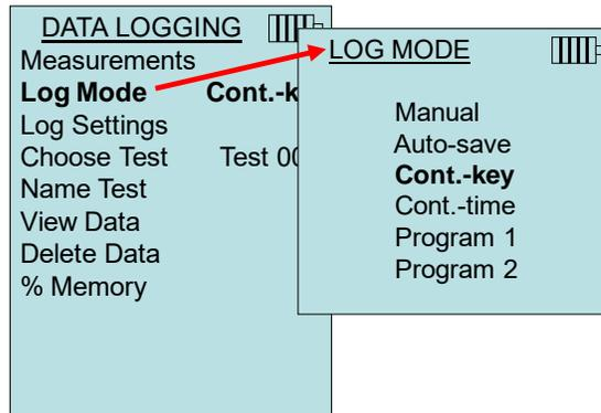
When set to Cont. key, the log interval can be adjusted.
