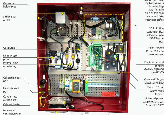
Up to 10 switching biogas inlets (time sharing) with fail-safe shut of solenoid valve and flow
