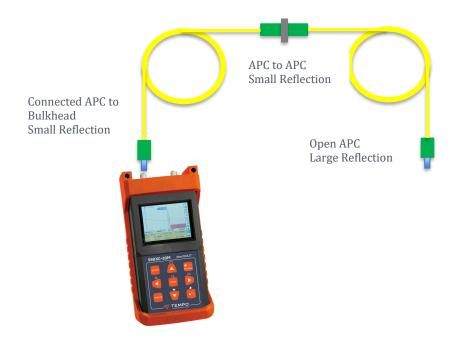
Mated APC connections have very low reflectivity (<65dB typical) An open (not connected) APC will have a high reflectivity (~45dB)
